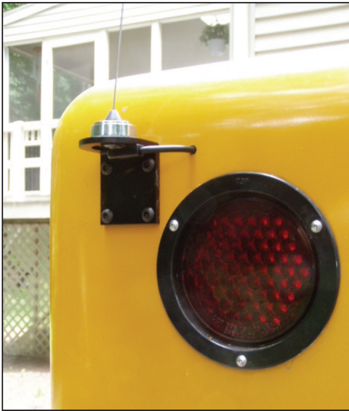
Above left: Exterior mounting of Type B antenna; Right: interior view of same antenna. Not the ground wire which is important to performance with a fiberglass cab. Below: A waterproof external speaker is very useful at rest stops.
